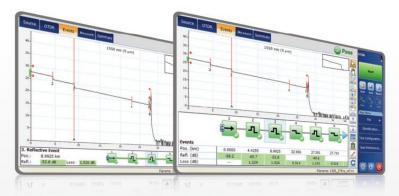
This improved linear view offers you the flexibility to display both the OTDR graph and its linear view without having to perform a toggle to analyze your fiber link.
