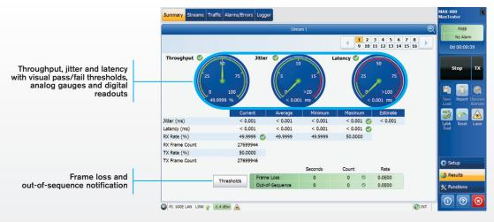
The analog gauges are lined with green and red regions to represent the expected thresholds.
