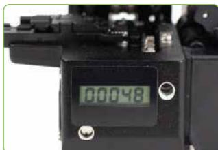
Cleave counts are indicated in real-time in a digital format.
