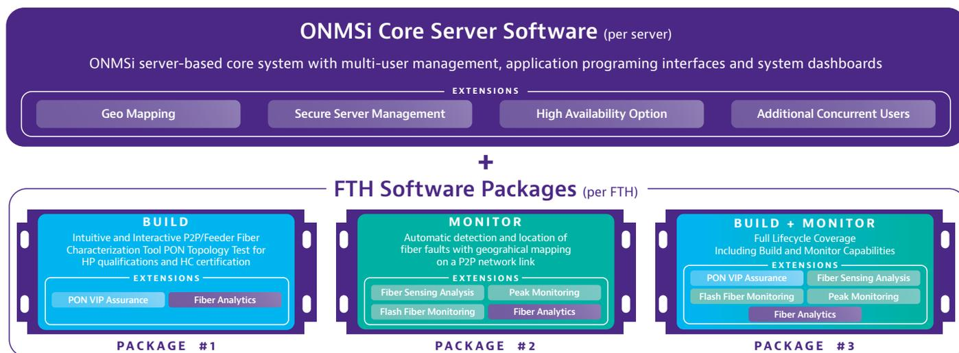
The ONMSi Core Server applies system wide and is administered from the central network server. Applications (Build, Monitor, or Combo) and extensions, such as Fiber Sensing Analysis apply to specific FTHs to allow specialized teams to select functionality they need for tasks such as construction or maintenance.
